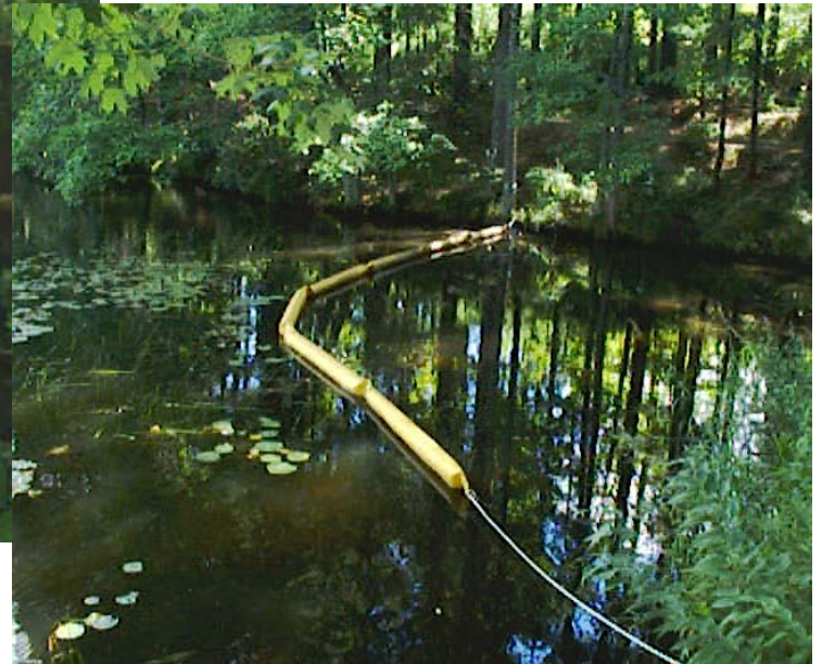
Figure 2-10. Floating Silt Boom that has Created the Sediment Delta.
